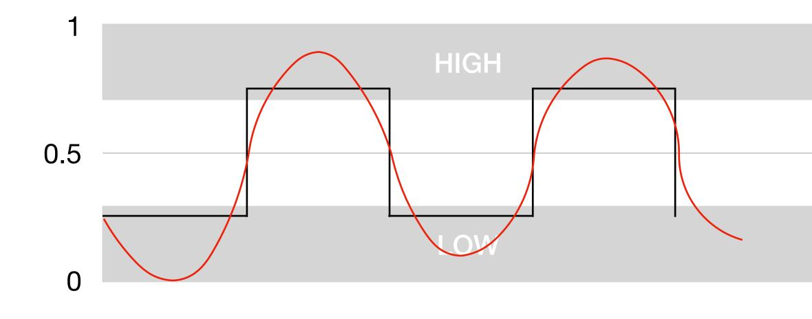
Voltage is still continuous in digital circuits
