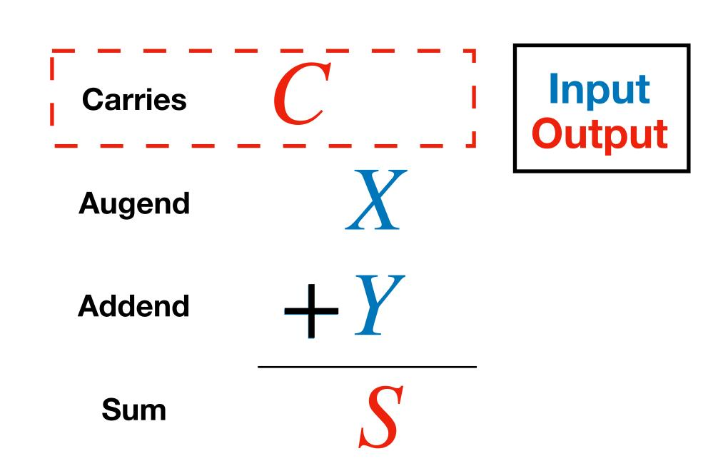
• Half adder input X, Y output S, C
