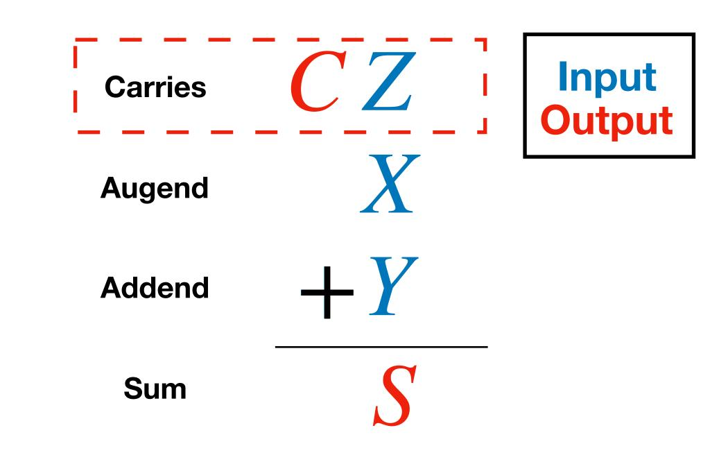
• Full adder input X, Y, Z; output S, C
