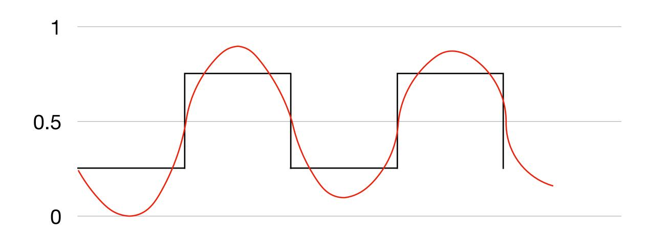
Voltage is still continuous in digital circuits
