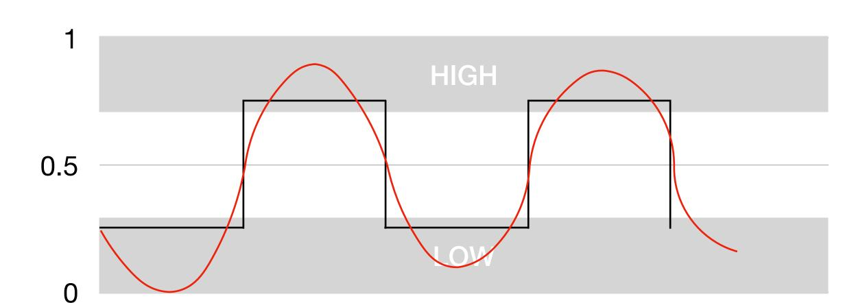
Voltage is still continuous in digital circuits
