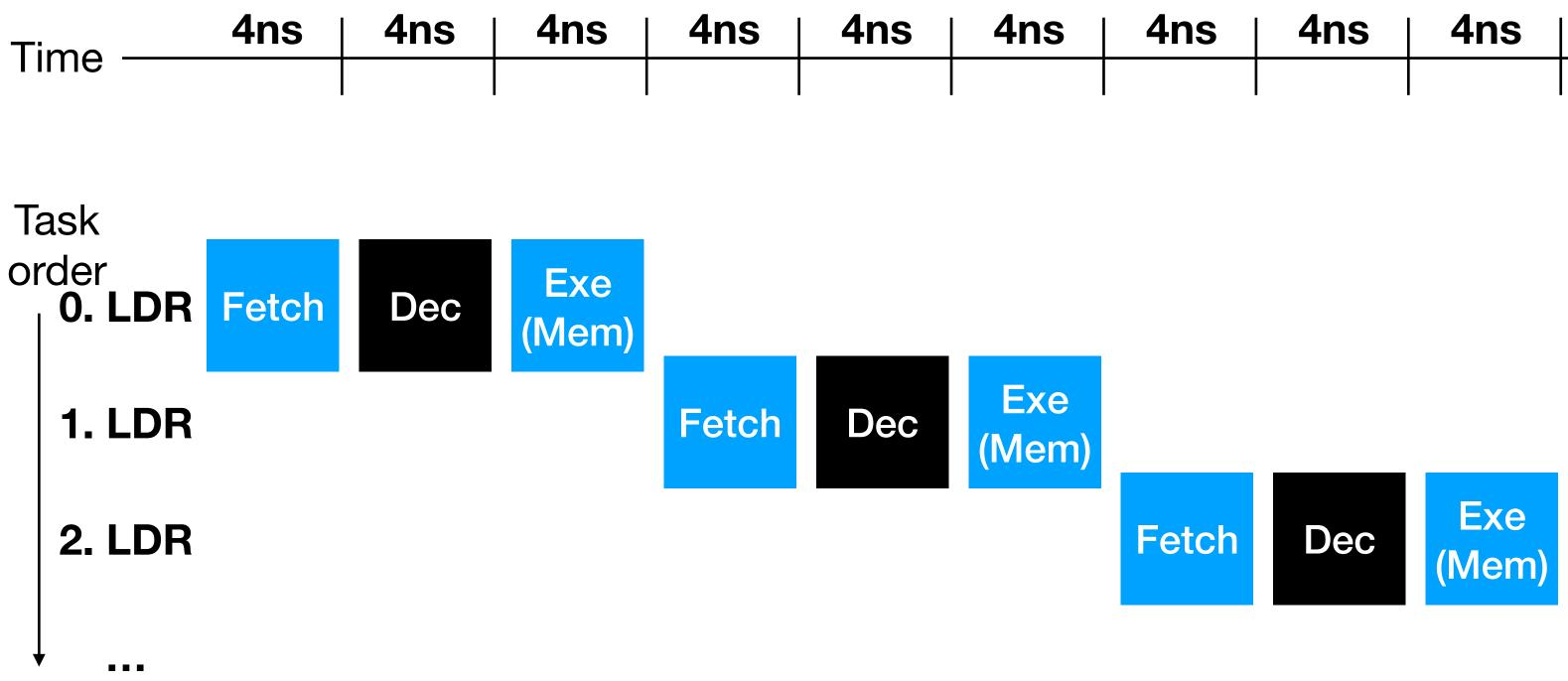
• Exe stages with memory operations cannot overlap with **Fetch**, decode however is fine
