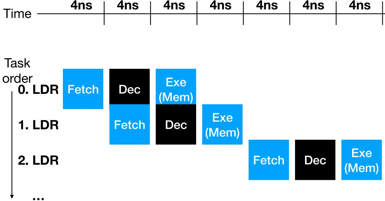
• Exe stages with memory operations cannot overlap with **Fetch**, decode however is fine (time reduction:  $1 \times 4ns = 4 ns$ )
