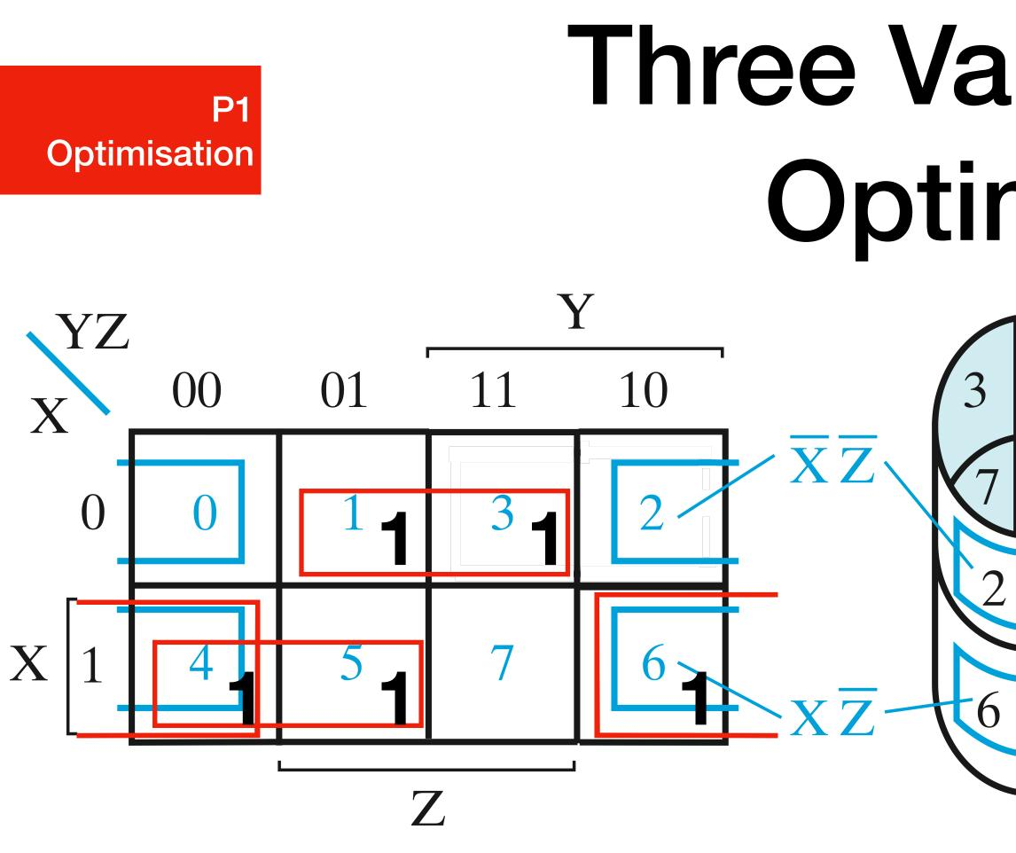
$F(X, Y, Z) = \Sigma m(1, 3, 4, 5, 6)$  $= \overline{X}Z + X\overline{Y} + X\overline{Z}$
