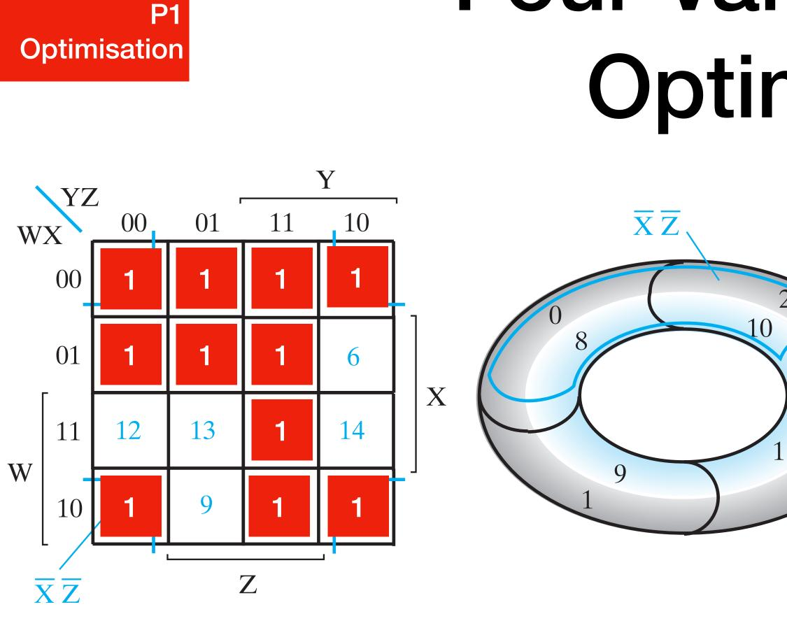
$F(W, X, Y, Z) = \overline{W}\overline{Y}\overline{Z} + \overline{W}Z + \overline{X}Y + YZ + W\overline{X}\overline{Z} \bullet$
