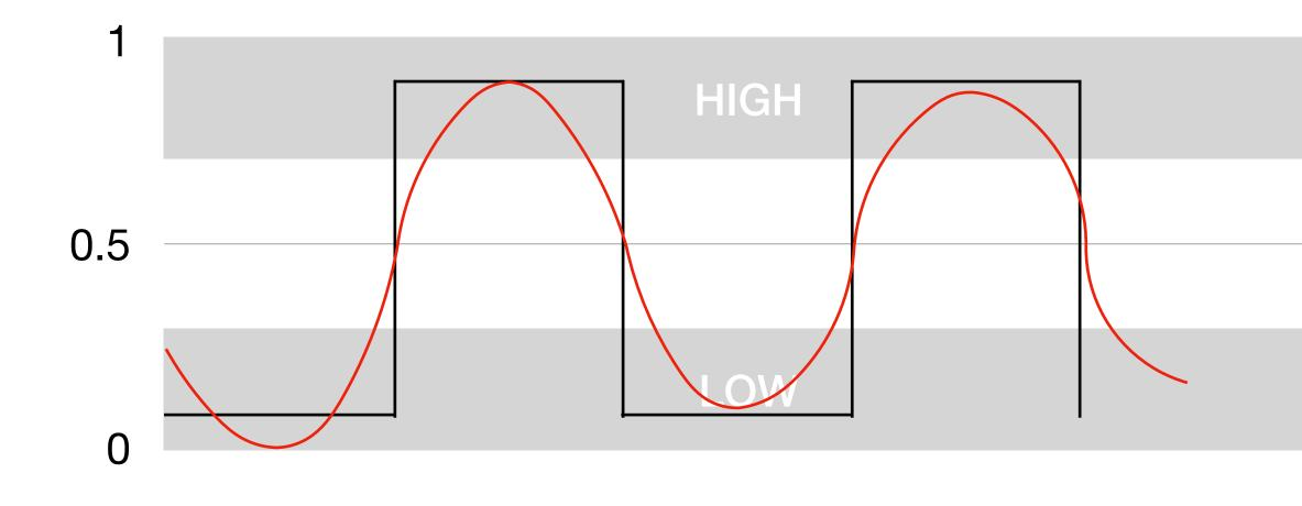
Voltage is still continuous in digital circuits
